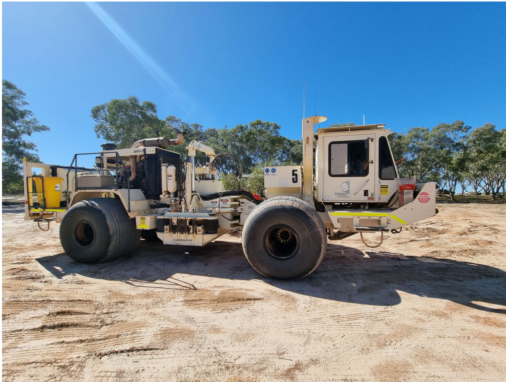
Figure 4: Seismic Vibroseis truck acquiring the Bookara 3D seismic survey
